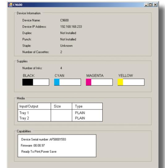
Bi-directional communication with printers to monitor status of the machine
